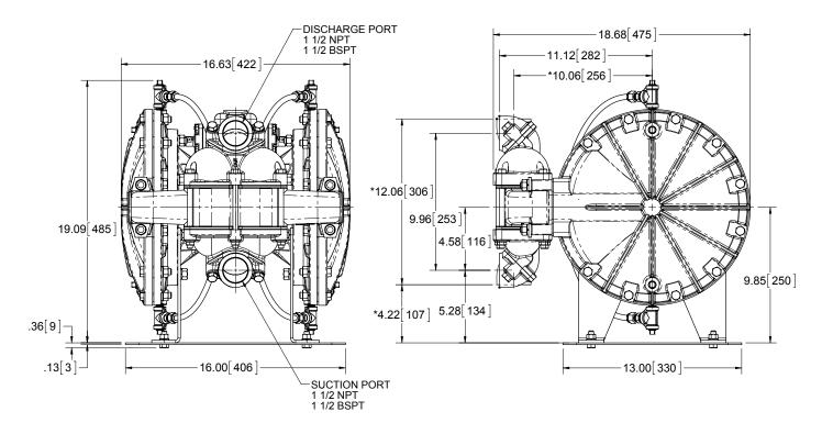
\* INDICATES DIMENSION WITH SUCTION AND DISCHARGE PORTS ROTATED 180° TO A VERTICAL POSITION
