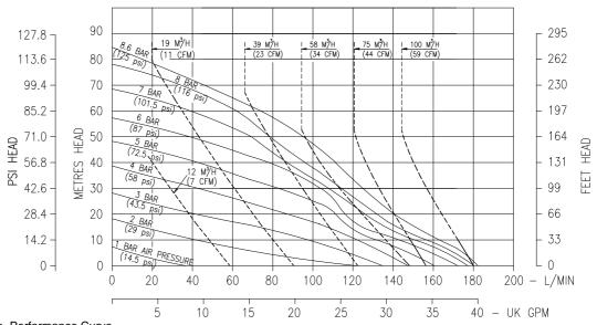
B2505 Metallic Pump, Performance Curve, based on water at ambient temperature
